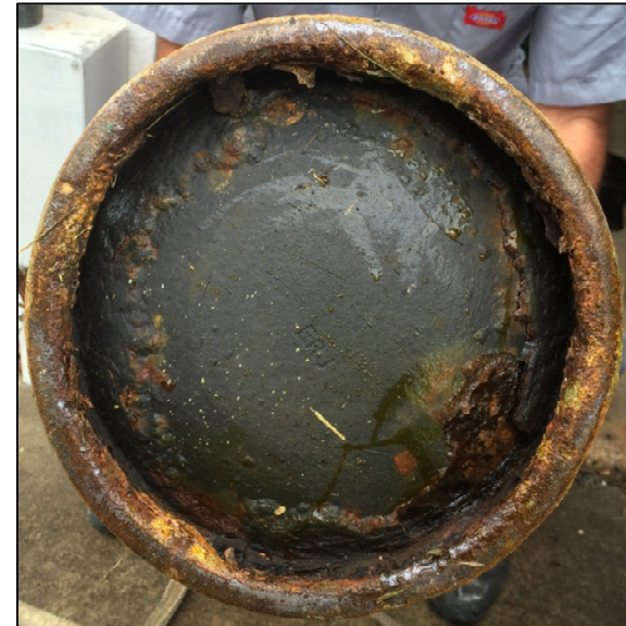
Bottom of Severely Corroded Chlorine Cylinder
