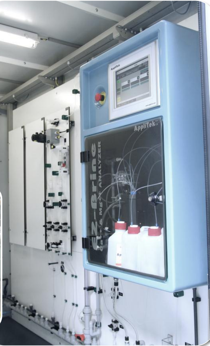
Thailand 29/02/2011 AnaShell® single-compartment protective shelter 1 x EZ-Brine® on-line Analyzer system for Ca ++ & Mg ++ in Ultra-purified brine
