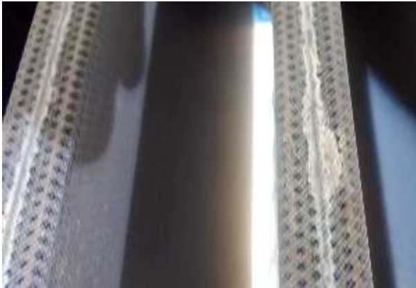
A nylon screen is installed on the cathode screen
