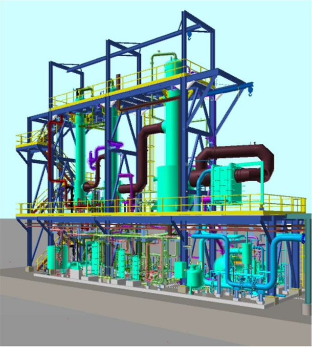
486 mtpd (as NaOH 100%) triple effect evaporation plant
