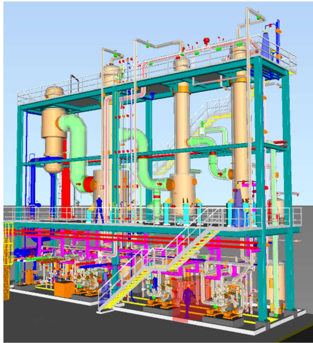
400 mtpd (as NaOH 100%) triple effect evaporation plant
