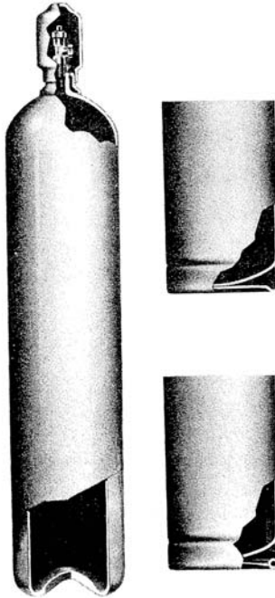
Figure 1 - Chlorine Cylinder (Left - bump-bottom; Upper right - double-bottom; Lower right - foot-ring)
